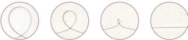
Nitinol "J" guidewires have kink-resistant properties
