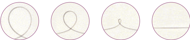
Nitinol "J" guidewires have kink-resistant properties
